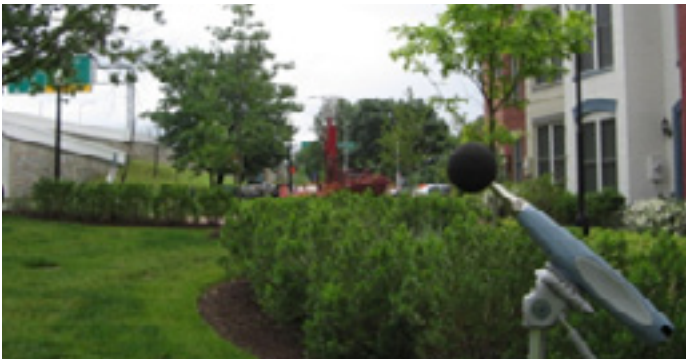
Sound level meters in operation along Virginia Avenue
